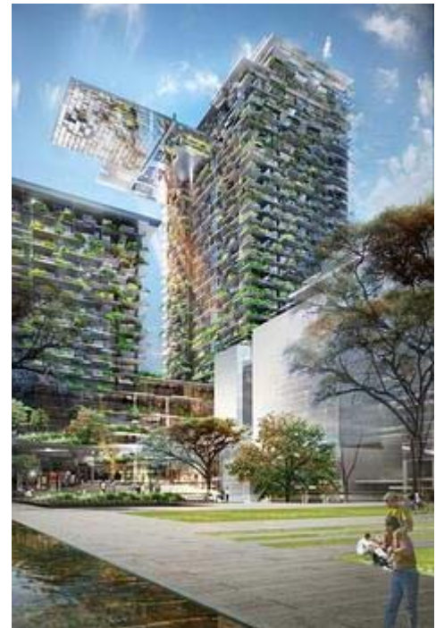
The Central Park tower with a heliostat to reflect light back into the apartments
